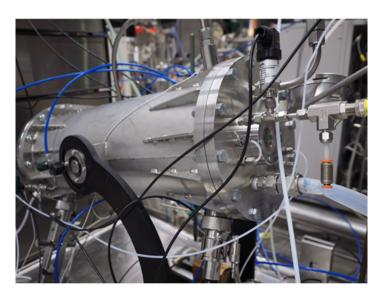
Figure 1: Gas fermentor (VTT 2020, LUT image bank)
